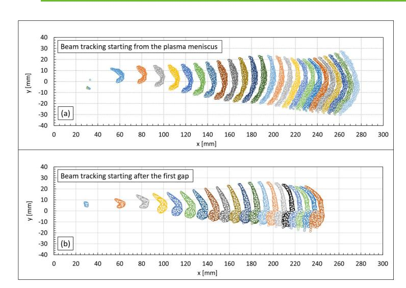
Shape of the accelerated bunches by their projection on the xy-plane, followed during 25 turns at moments when the RF phase equals zero
